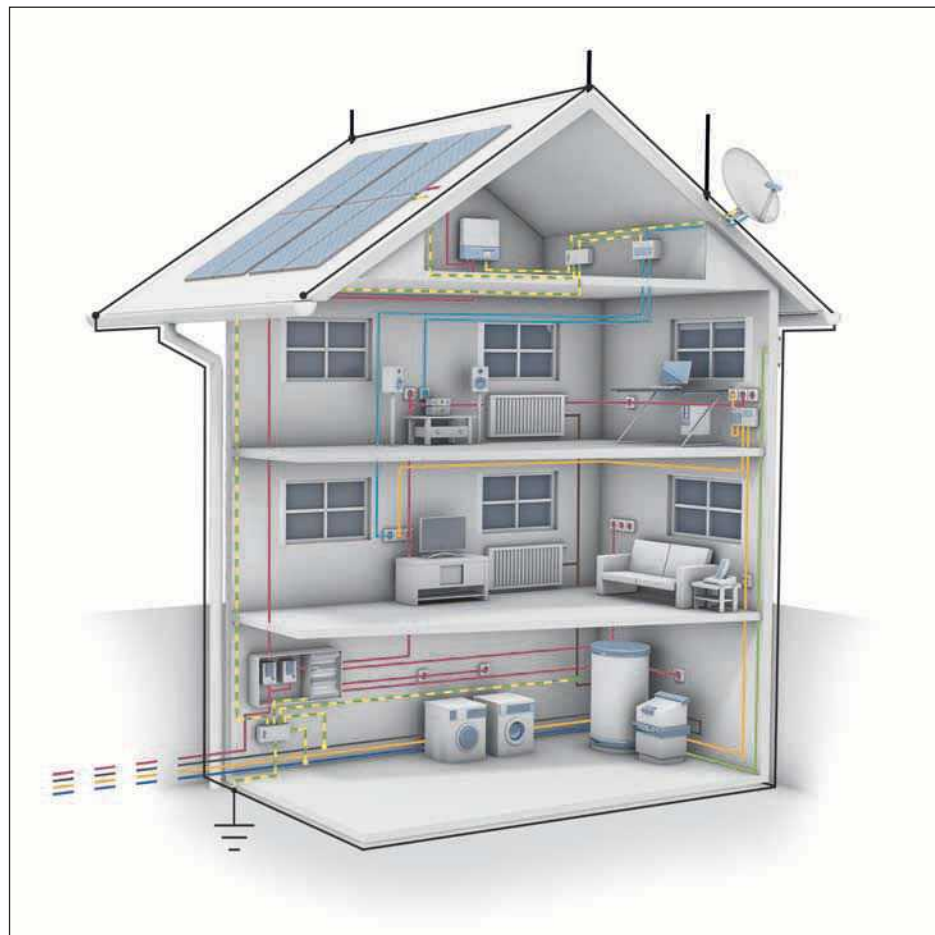
Fig. 68: Rooftop system on a single-family dwelling
