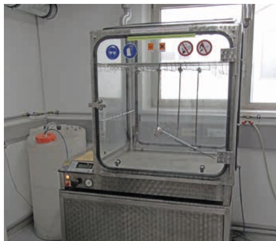
Figure 5.8.2 Test in a Kesternich chamber
