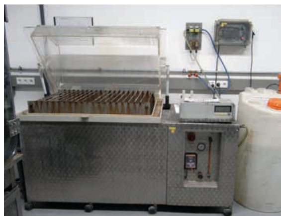
Figure 5.8.1 Test in a salt mist chamber
