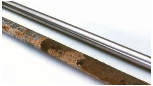
Figure 5.9.7 Corrosion of a galvanised earth rod (below) and a stainless steel earth electrode (above) after 2.5 years
