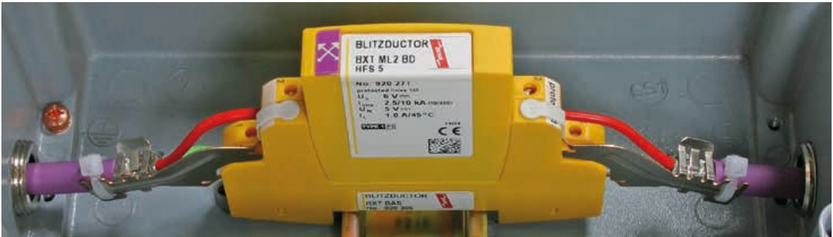
Figure 6.3.3 EMC spring terminals for the protected and unprotected side of a BLITZDUCTOR XT for permanent low-impedance shield contact with a shielded signal line; with snap-on insulating cap for indirect shield earthing, cable ties and insulating strips.
